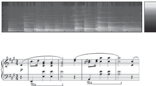
Fig. 25.6 Polyphonic music transcription. The task is to generate a human readable score as shown below, given the acoustic input. The computational problem here is to infer pitch, number of notes, rhythm, tempo, meter, time signature. The inference can be achieved online (filtering) or offline (smoothing), depending upon requirements.
